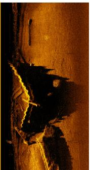
The above image of the *Betsy,* known as YO88 sunk in 1781, Yorktown River, was taken with the ARC Explorer Mk II using 1800 kHz transducers at a 30 m Range. The corrugated steel cofferdam is clearly visible around the wreck highlighted by the density of the steel. The less dense elongated concrete blocks protecting the top of the wreck resemble the ship's deck and can be distinguished from the steel.
