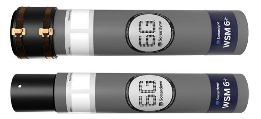
The Wideband®Sub-Mini 6+ (WSM 6+) is Sonardyne's latest generation of versatile Ultra-Short BaseLine (USBL) transponders/responders that support Wideband 2 signals. The WSM 6+ is designed for positioning Remotely Operated Vehicles (ROVs), towfish and other mobile targets in water depths up to 4,000 m.
